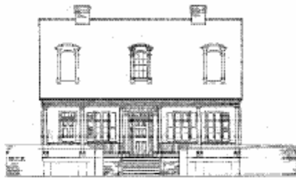
Creole Cottage – End gable with porches under main roof
